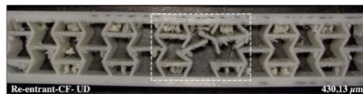
Figure 4.62 Re-entrant sandwich structure reinforced with CF containing a UD lay-up, showing the vicinity of damage after a CAI test
