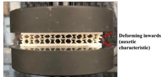
Figure 4.17 Auxetic behaviour indication from re-entrant cells
