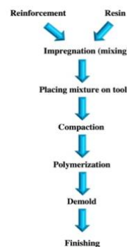
Figure 2.12 Conventional manufacturing method for fibre reinforced polymer composites (Nagavally, 2016)
