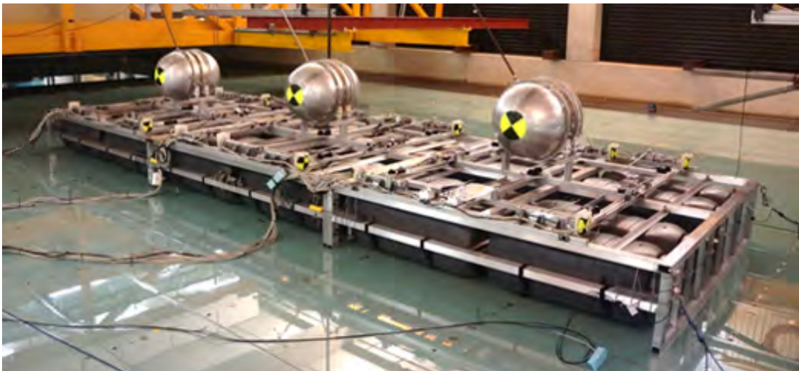
Figure 4.2: Multi-float device shown here in 3D horizontal float spacing before tank floor lowered for testing. Taken during May/June 2017 testing period.
