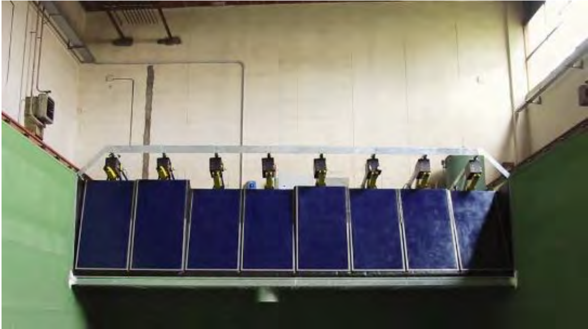
Figure 2.13: Wave maker at University of Naples [95].
